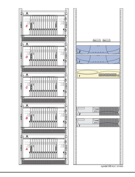
The left data rack contains a stack of five G650 Media Gateways that are labeled A through E. The right data rack contains the following (from top to bottom):
